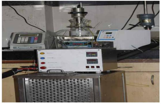
Acoustic cavitation set-up
