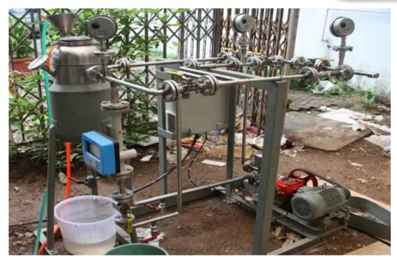
Hydrodynamic Cavitation Set-up
